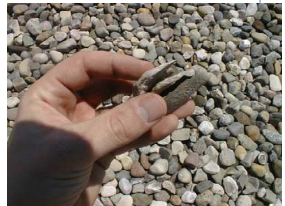
Sharp edges observed at the shaling ballast.
